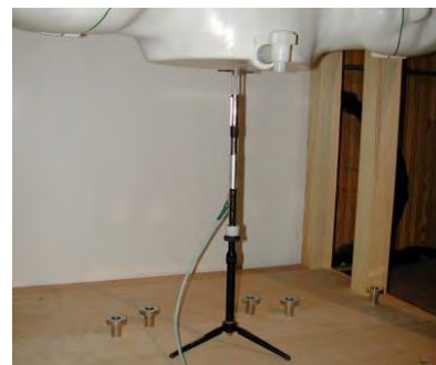
Figure 10-2 System Verification Setup Photo
