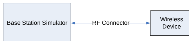
Figure 9-2 Power Measurement Setup
