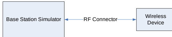
Figure 9-1 Power Measurement Setup
