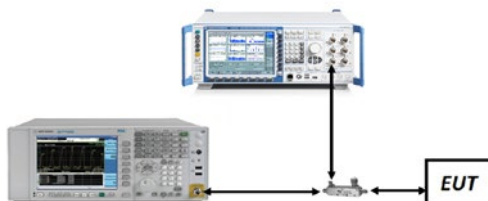
Figure 7-2. Test Instrument & Measurement Setup
