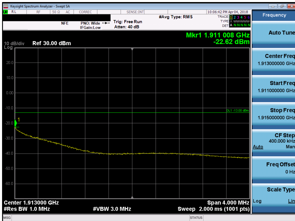
Plot 7-76. 4MHz Span Plot (PCS CDMA Mode - High Channel)
