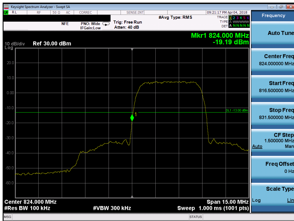
Plot 7-77. Band Edge Plot (Cellular WCDMA Mode - Low Channel)
