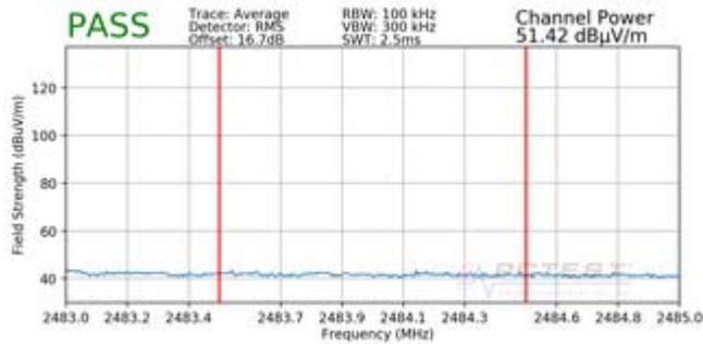
Plot 7-37. Radiated Restricted Upper Band Edge Measurement (Average)
