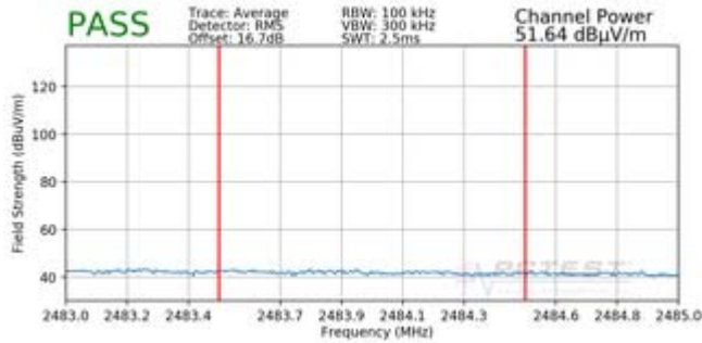
Plot 7-39. Radiated Restricted Upper Band Edge Measurement (Average)
