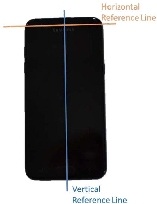
SAR Test Setup Photo 12: Vertical and Horizontal Reference Lines
