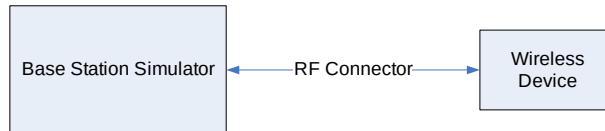
Figure 9-1 Power Measurement Setup
