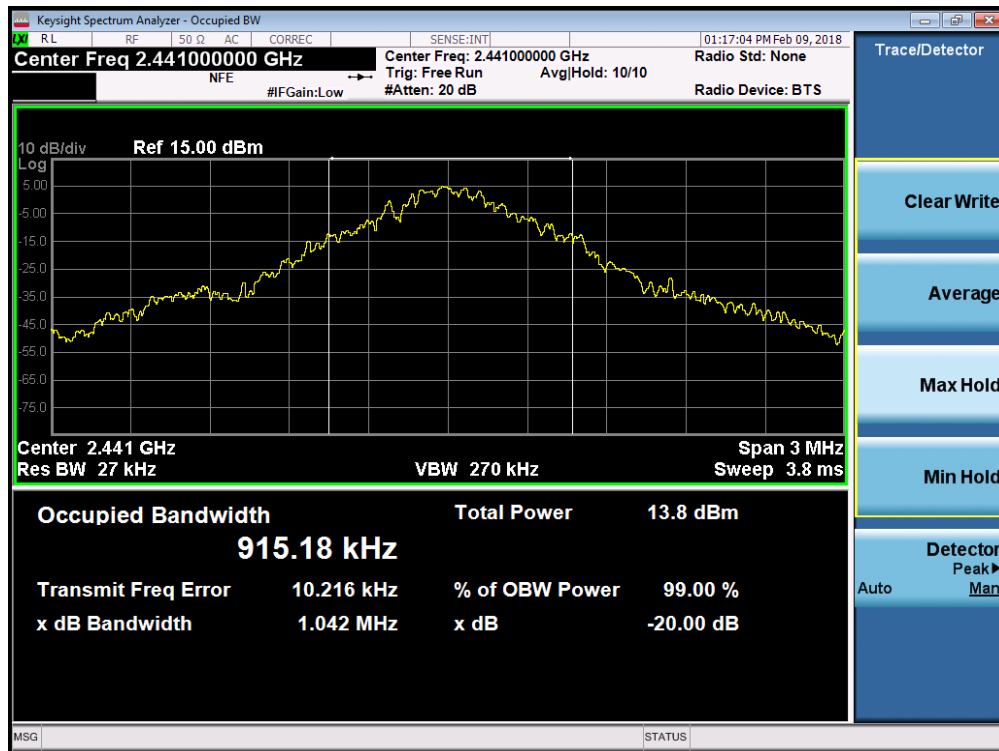
Plot 7-2. 20dB Bandwidth Plot (Bluetooth, 1Mbps – Ch. 39)
