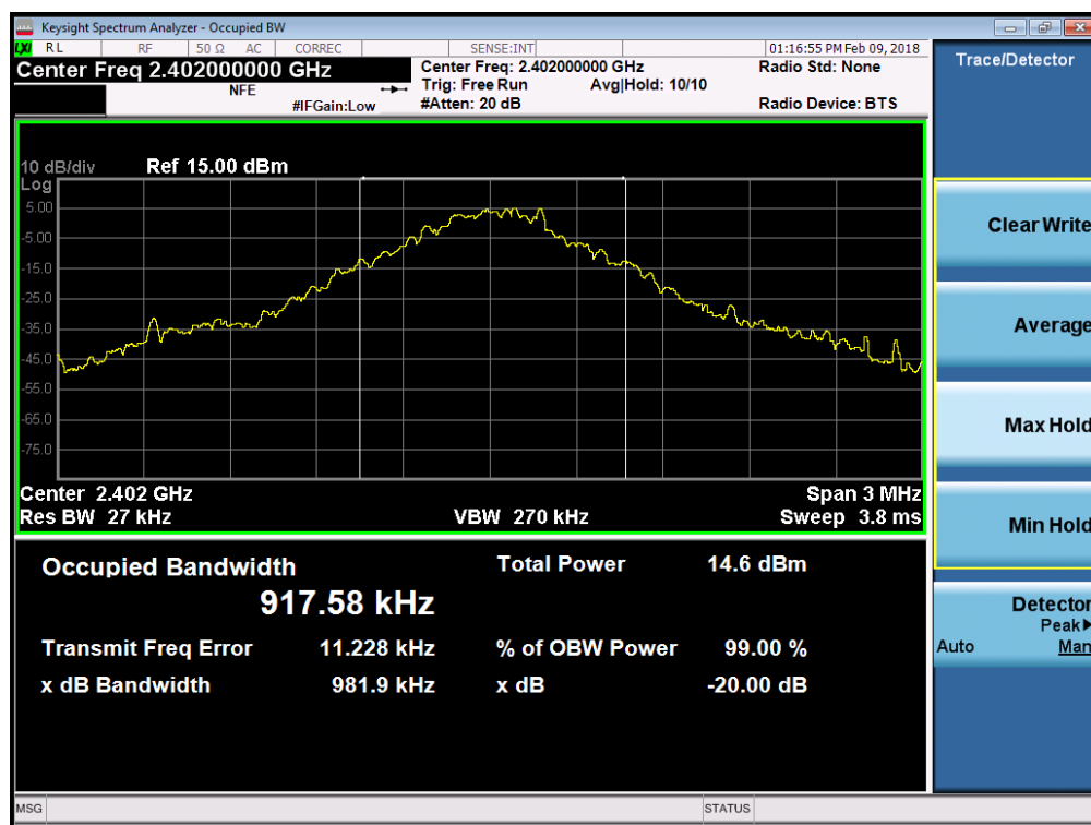
Plot 7-1. 20dB Bandwidth Plot (Bluetooth, 1Mbps – Ch. 0)
