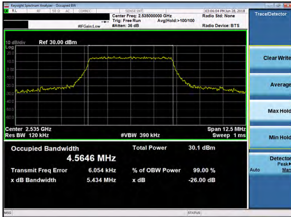
Plot 7-41. Occupied Bandwidth Plot (Band 7 - 5.0MHz QPSK - Full RB Configuration)
