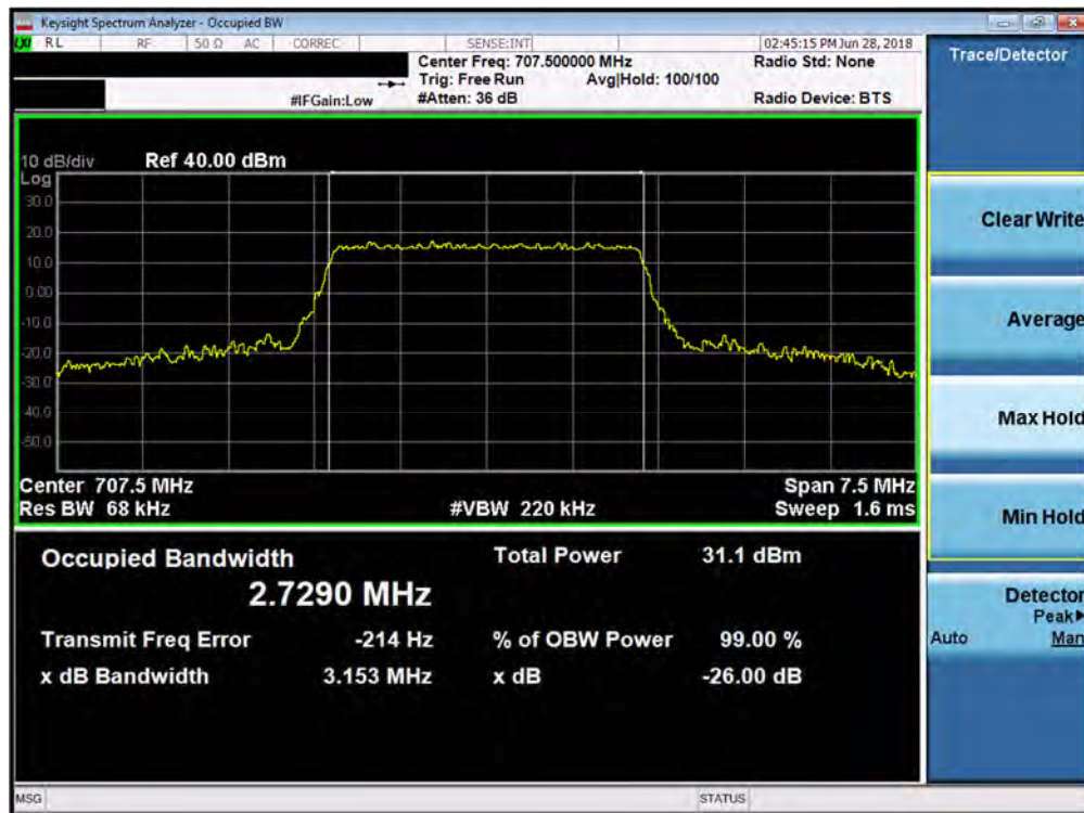
Plot 7-4. Occupied Bandwidth Plot (Band 12 - 3.0MHz 16-QAM - Full RB Configuration)
