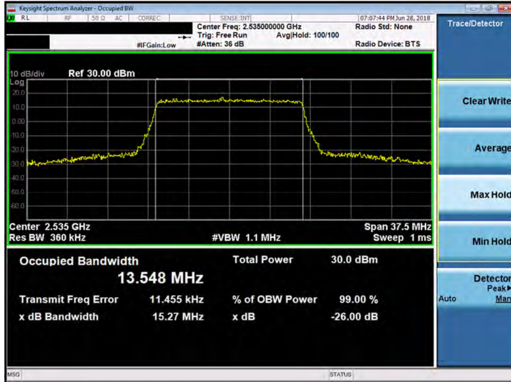
Plot 7-45. Occupied Bandwidth Plot (Band 7 - 15.0MHz QPSK - Full RB Configuration)
