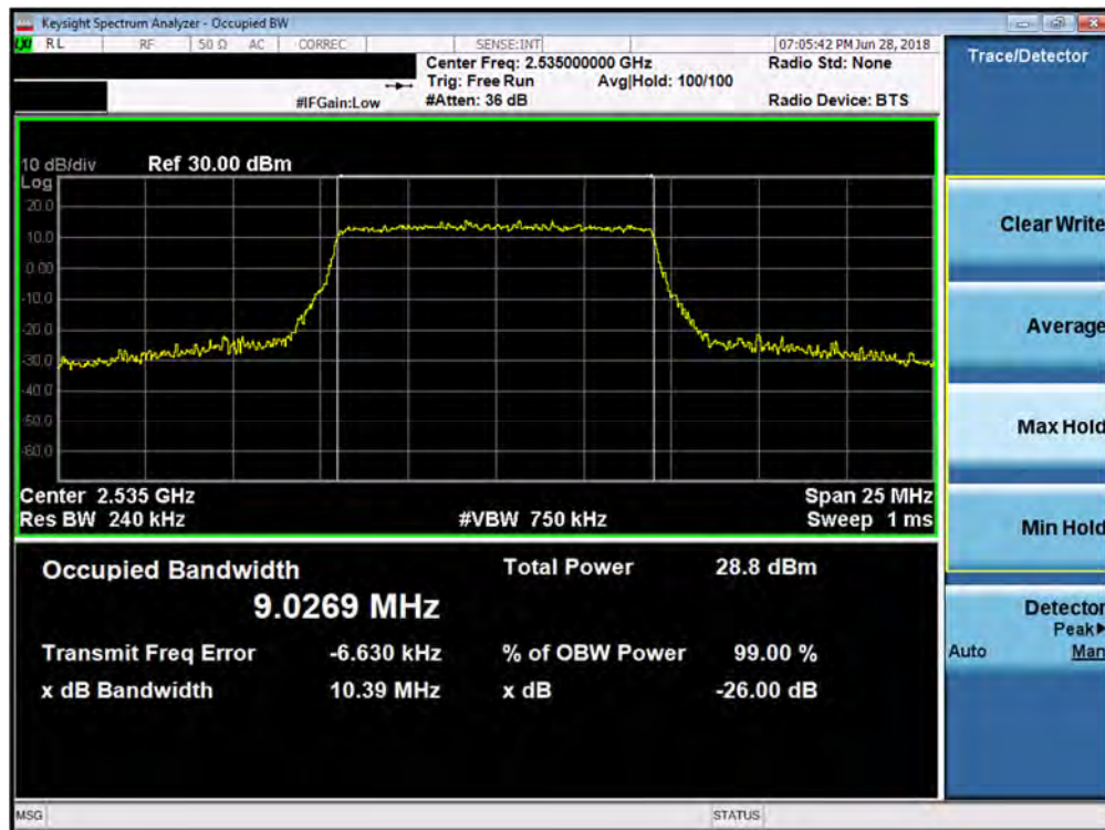
Plot 7-44. Occupied Bandwidth Plot (Band 7 - 10.0MHz 16-QAM - Full RB Configuration)
