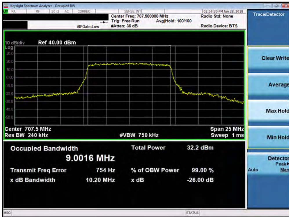
Plot 7-7. Occupied Bandwidth Plot (Band 12/17 - 10.0MHz QPSK - Full RB Configuration)
