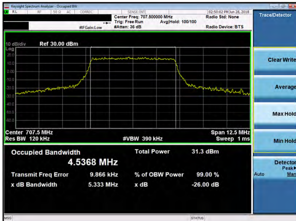
Plot 7-6. Occupied Bandwidth Plot (Band 12/17 - 5.0MHz 16-QAM - Full RB Configuration)
