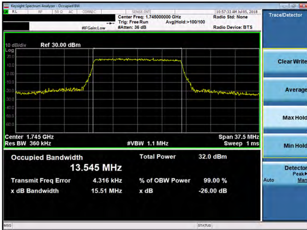
Plot 7-25. Occupied Bandwidth Plot (Band 66/4 - 15.0MHz QPSK - Full RB Configuration)
