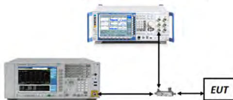
Figure 7-3. Test Instrument & Measurement Setup
