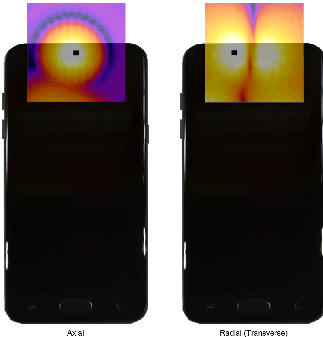
Axial Radial (Transverse) Figure 16-3 T-Coil Scan Overlay Magnetic Field Distributions
