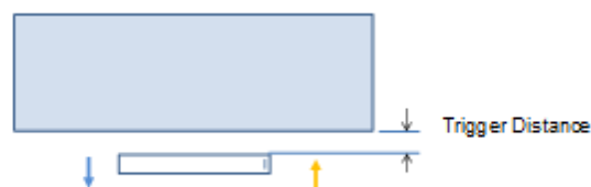
Proximity Sensor Trigger Distance Assessment KDB 616217 §6.2, Front
