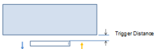
Proximity Sensor Trigger Distance Assessment KDB 616217 §6.2, Front
