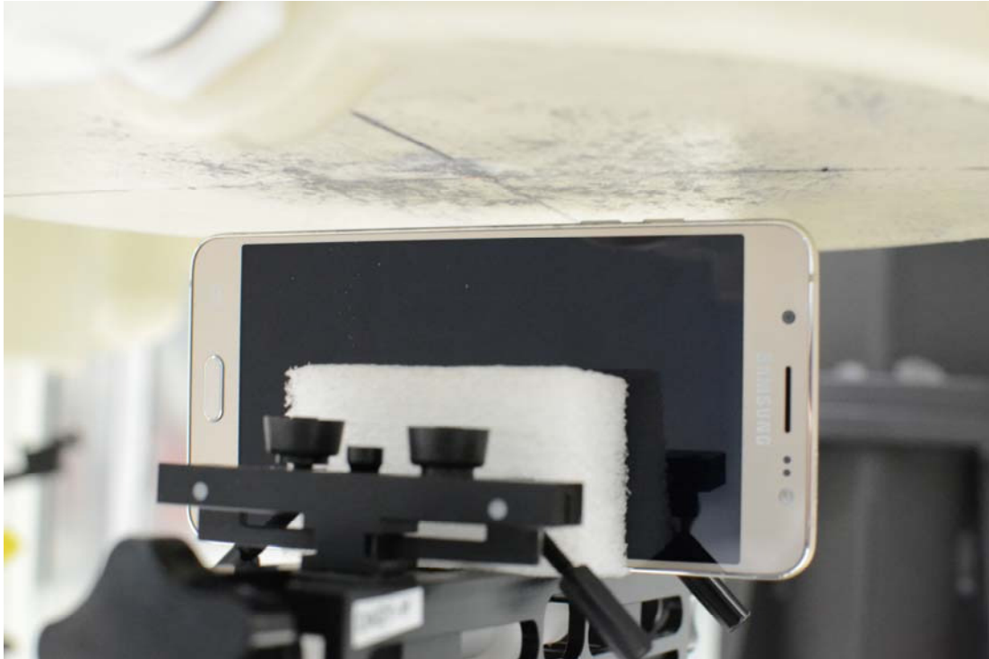
SAR Test Setup Photo 13: Left at 1.0 cm
