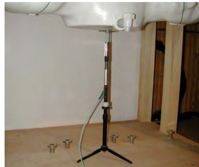
Figure 10-2 System Verification Setup Photo
