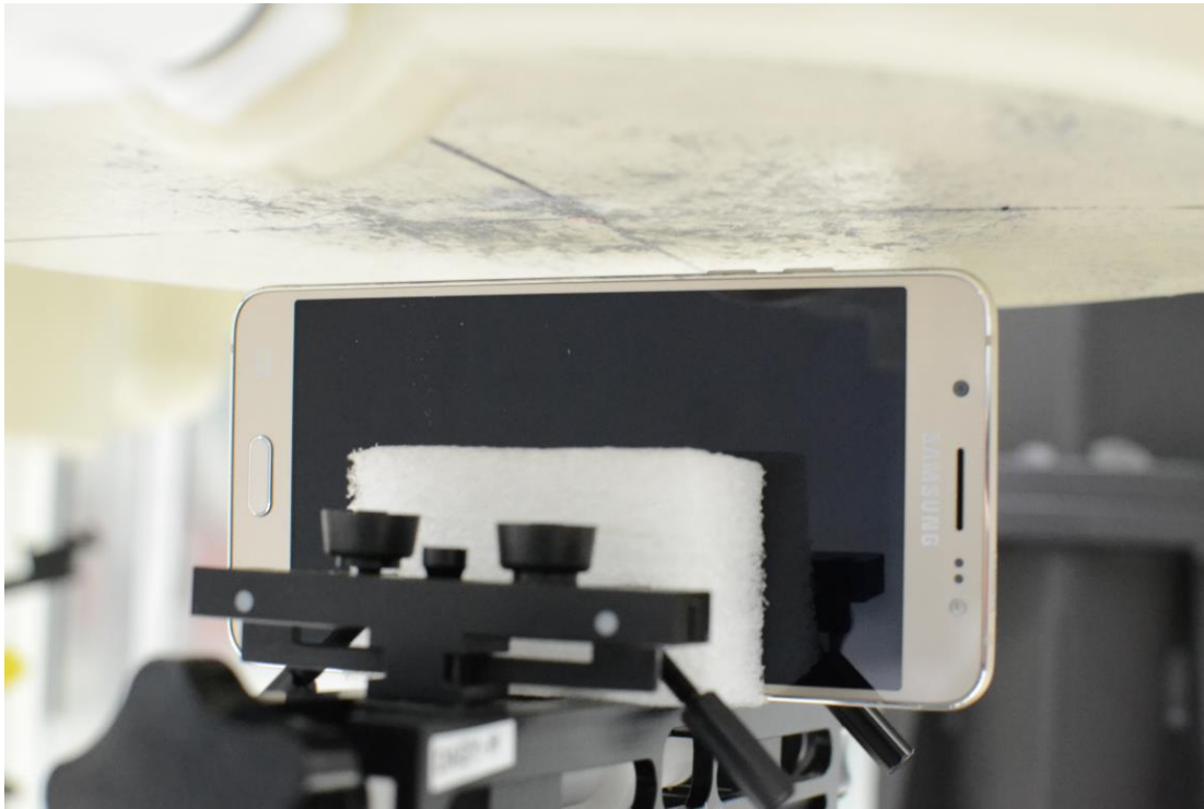
SAR Test Setup Photo 11: Left at 1.0 cm
