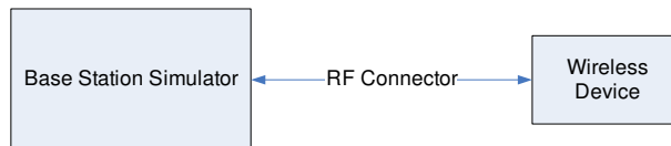
Figure 9-1 Power Measurement Setup
