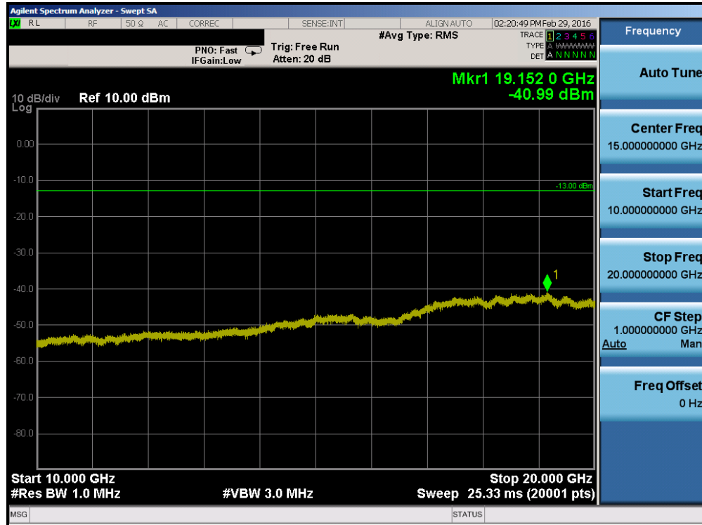
Plot 7-40. Conducted Spurious Plot (AWS WCDMA Mode – Ch. 1412)
