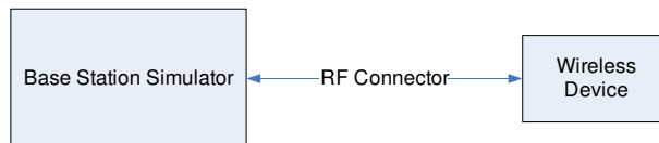
Figure 9-2 Power Measurement Setup
