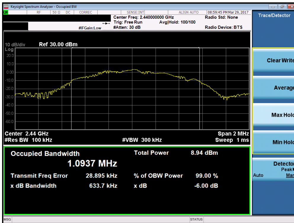
Plot 7-2. 6dB Bandwidth Plot (Bluetooth (LE) – Ch. 19)
