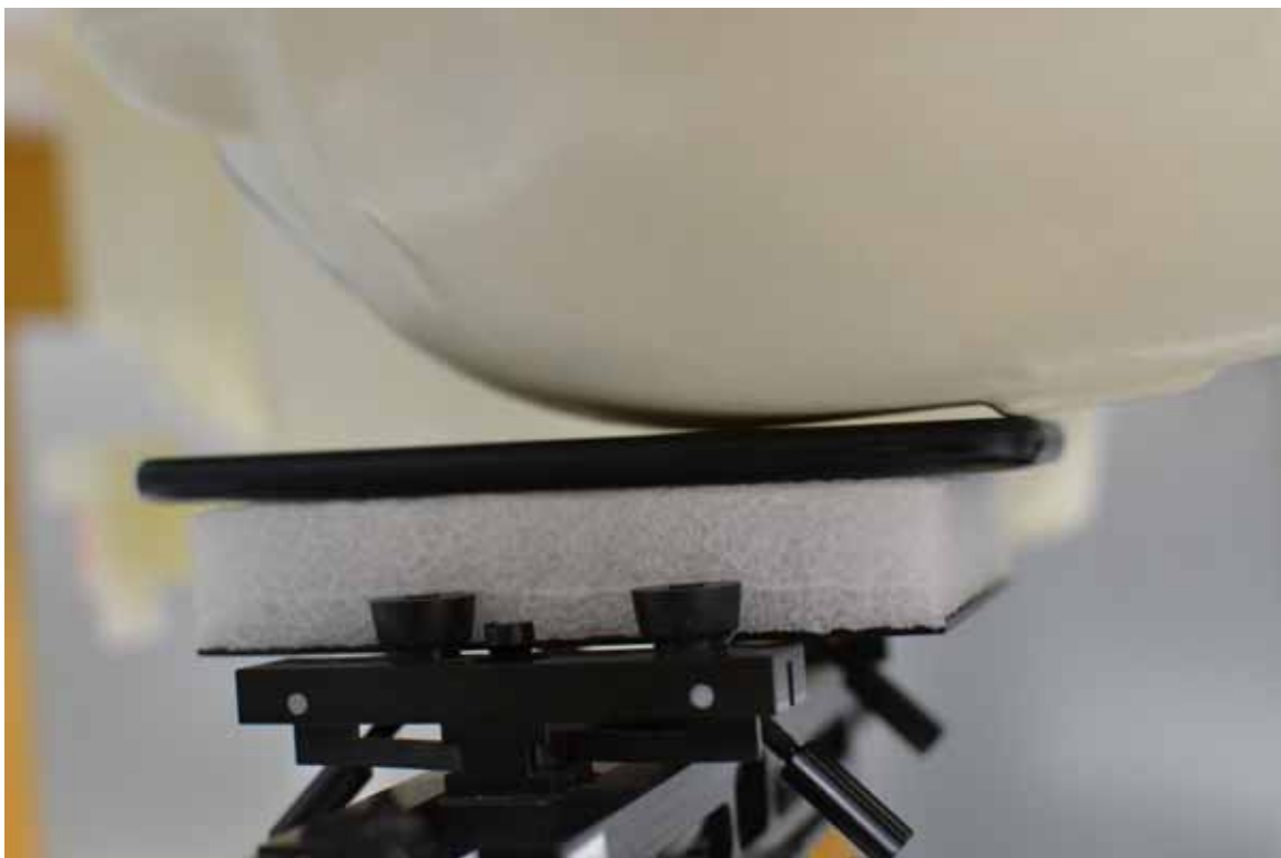
SAR Test Setup Photo 3 – Left Cheek
