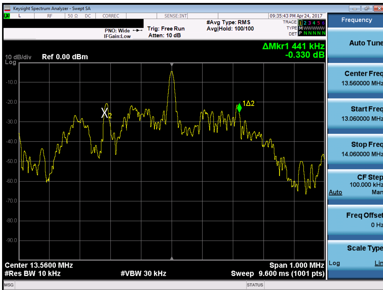
Figure 8-2. 20dB Bandwidth Plot
