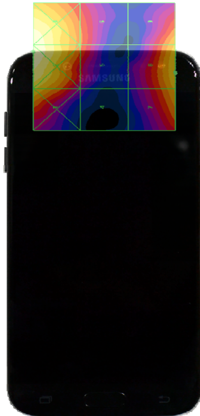
Figure 17-4 E-Field WD Scan overlay
