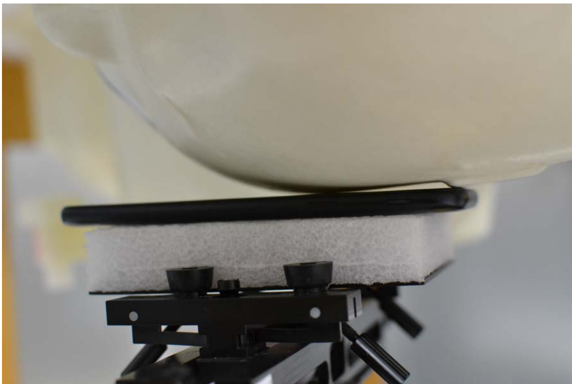
SAR Test Setup Photo 3 – Left Cheek
