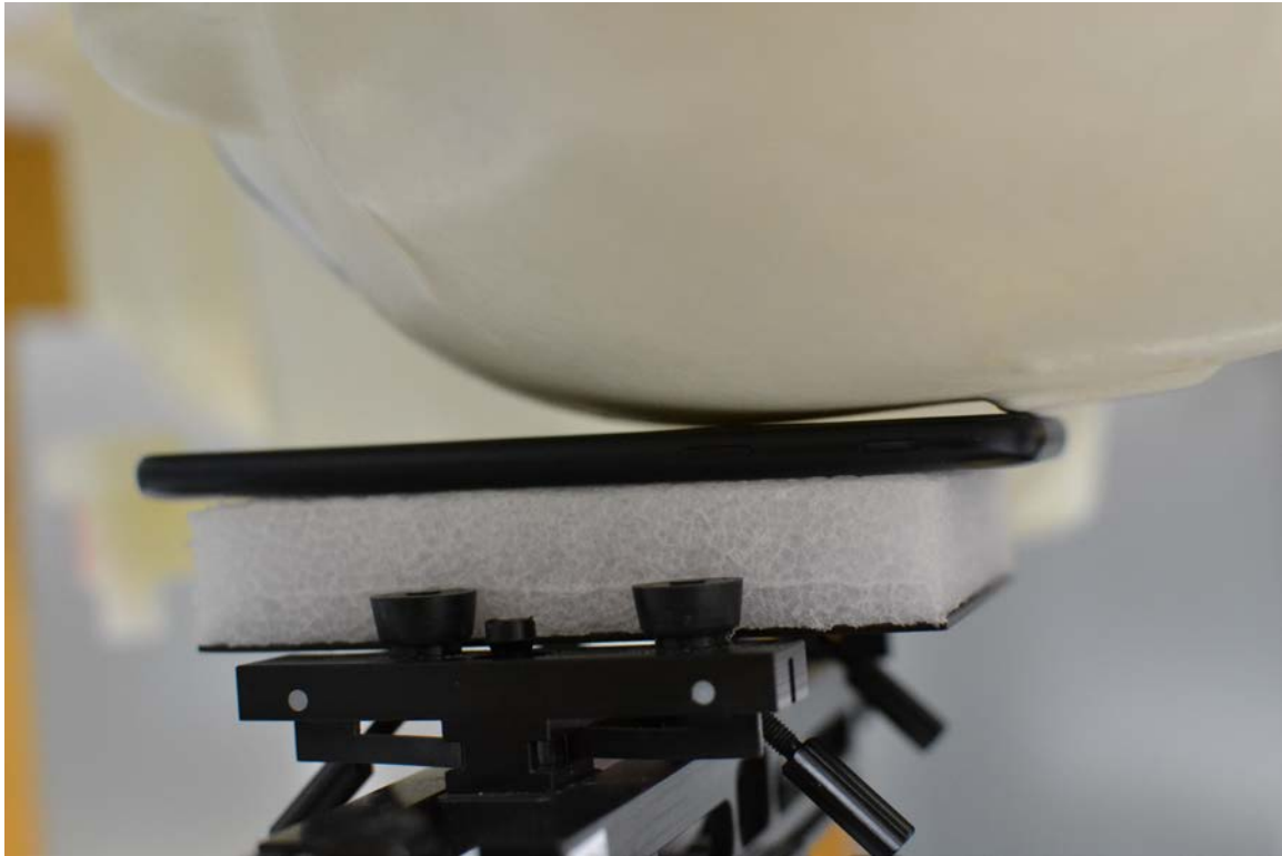
SAR Test Setup Photo 3 – Left Cheek
