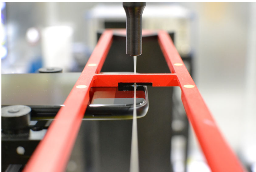
Figure 17-2 HAC Phantom Plane Alignment
