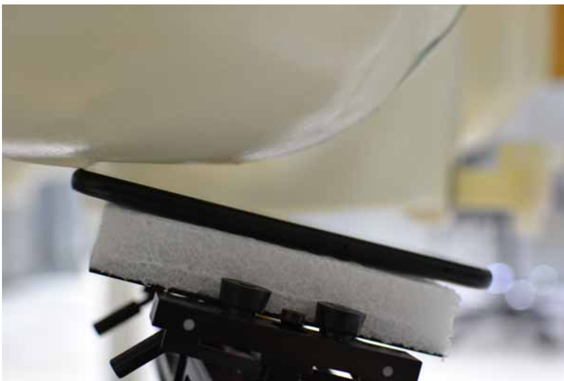
SAR Test Setup Photo 2 – Right Tilt
