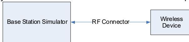
Figure 9-3 Power Measurement Setup
