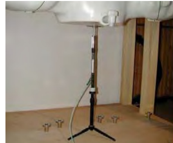
Figure 10-2 System Verification Setup Photo
