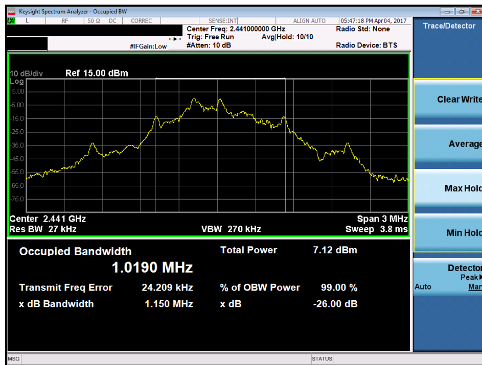
Plot 7-1. Occupied Bandwidth Plot (ANT+ – Ch. 39)
