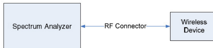
Figure 7-1. Test Instrument & Measurement Setup
