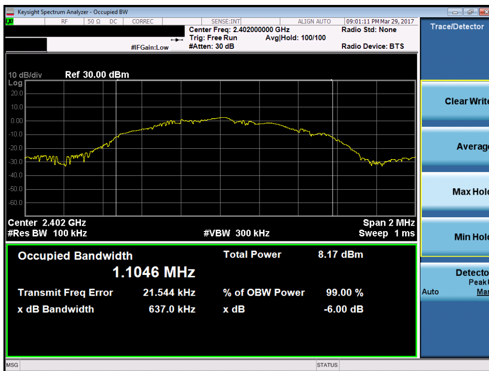
Plot 7-1. 6dB Bandwidth Plot (Bluetooth (LE) – Ch. 0)
