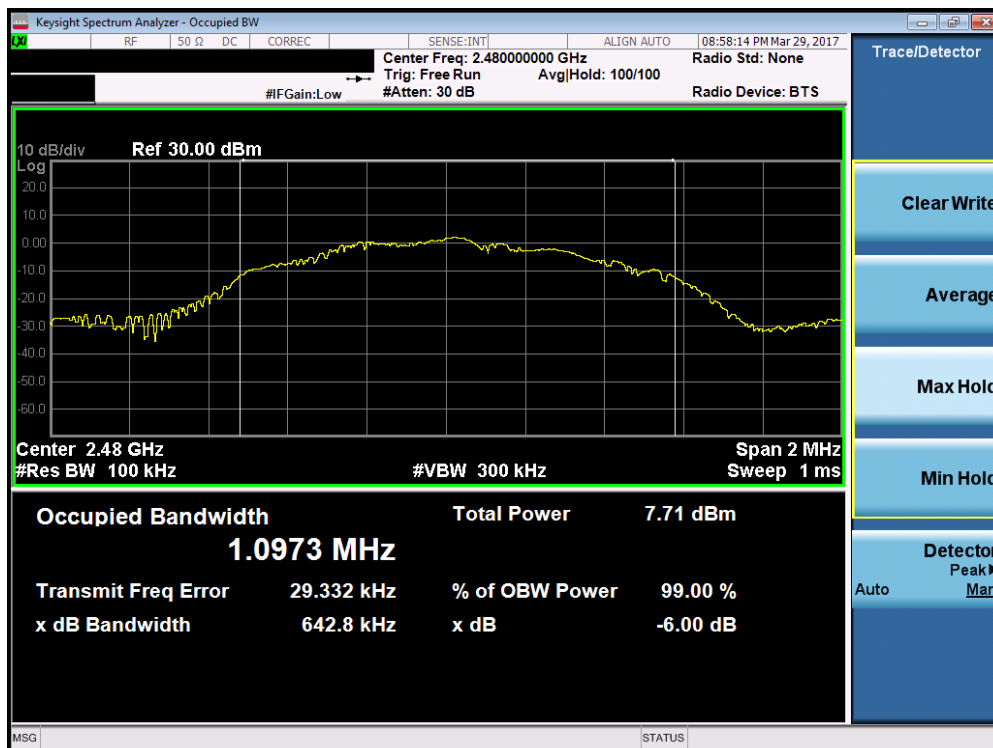
Plot 7-3. 6dB Bandwidth Plot (Bluetooth (LE) – Ch. 39)
