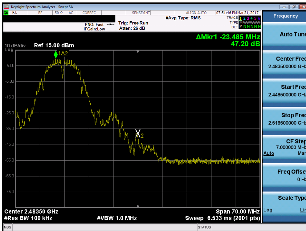
Plot 7-20. Band Edge Plot (802.11b – Ch. 11)
