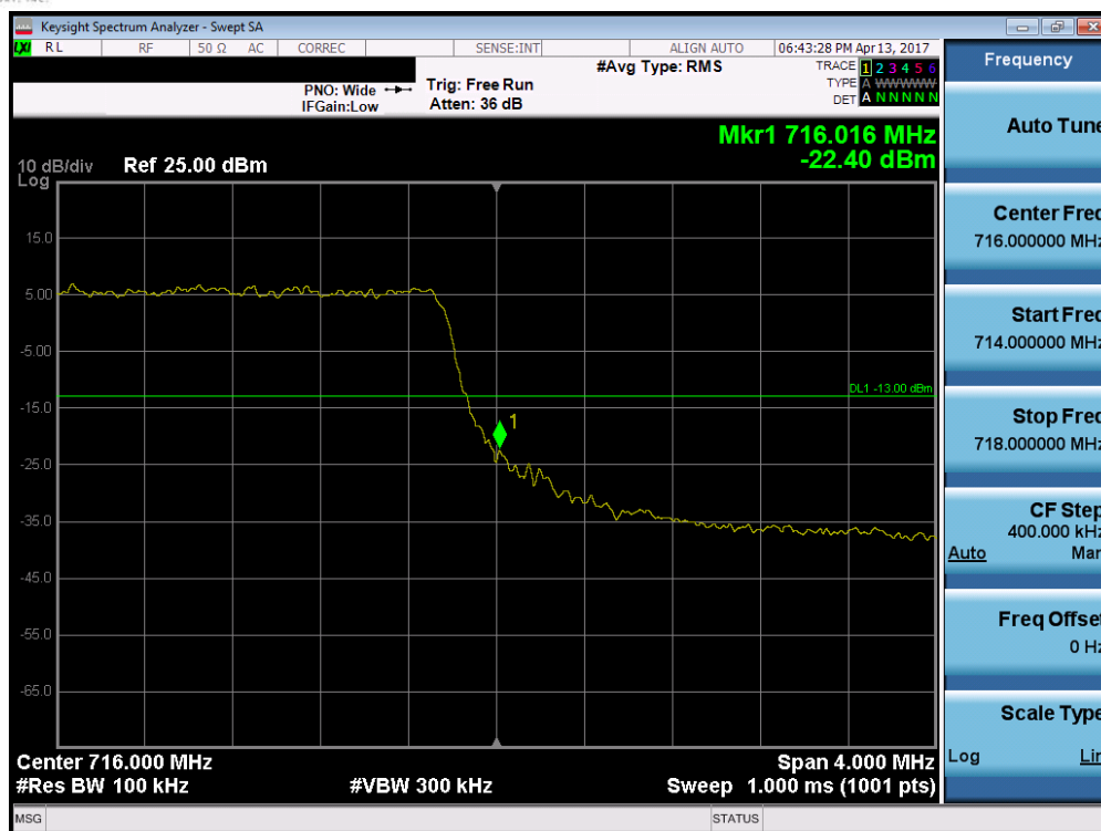
Plot 7-99. Upper Band Edge Plot (Band 12/17 – 5.0MHz QPSK – RB Size 25)
