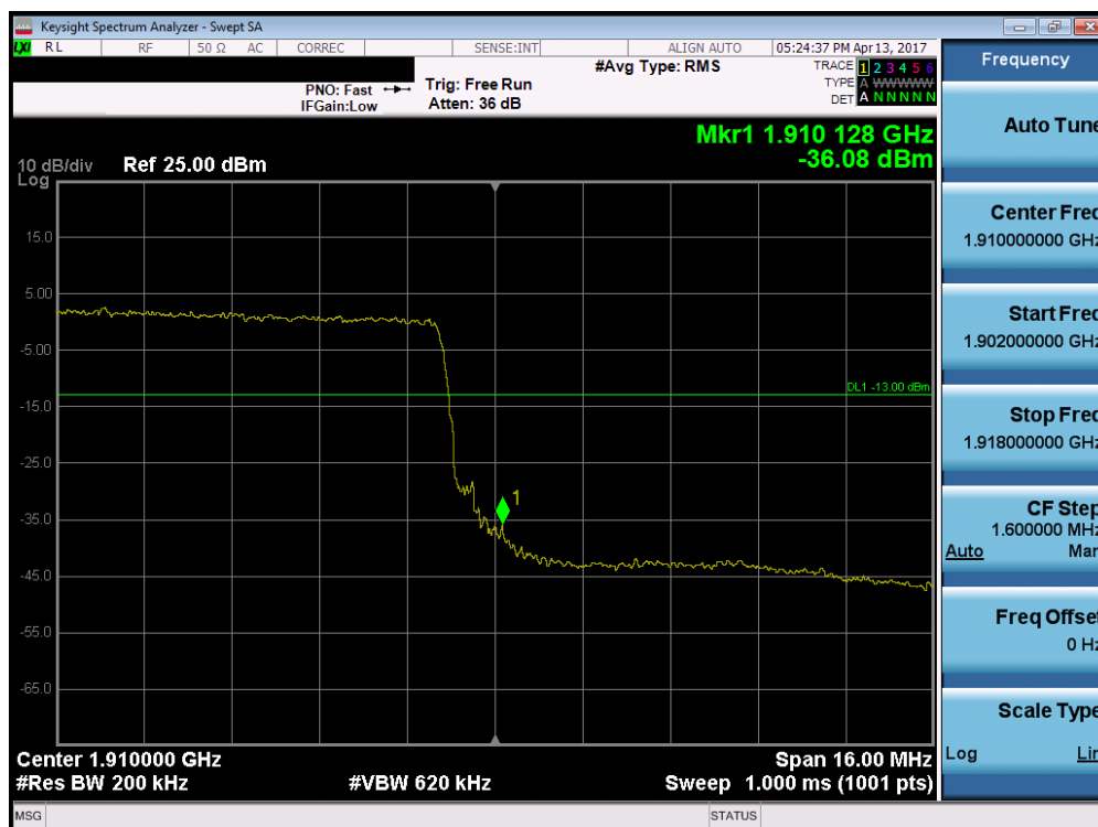
Plot 7-158. Upper Band Edge Plot (Band 2 – 20.0MHz QPSK – RB Size 100)
