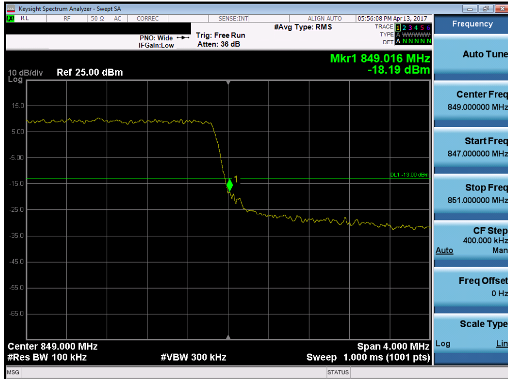
Plot 7-107. Upper Band Edge Plot (Band 5 – 3.0MHz QPSK – RB Size 15)
