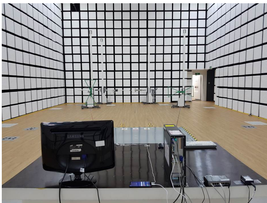
[ Radiated Disturbance for Below 1 GHz – Rear ]
