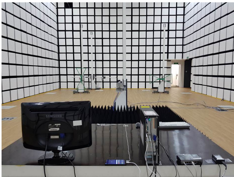
[ Radiated Disturbance for Above 1 GHz – Rear ]
