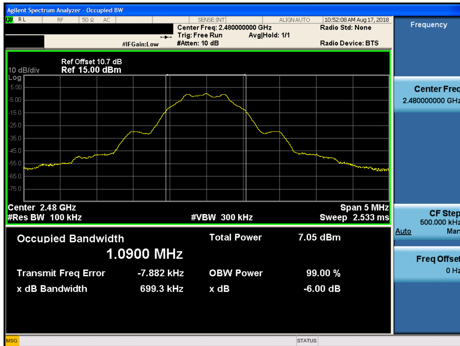
6 dB Bandwidth plot (High-CH 39)
