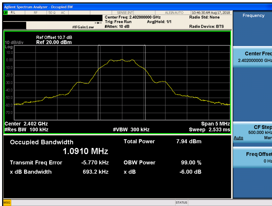
6 dB Bandwidth plot (Low-CH 0)
