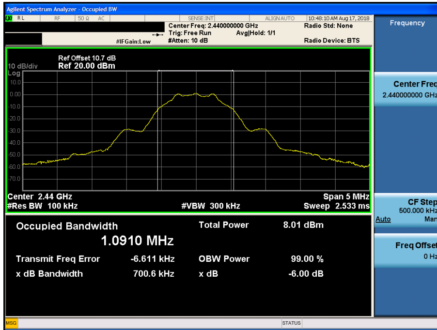
6 dB Bandwidth plot (Mid-CH 19)
