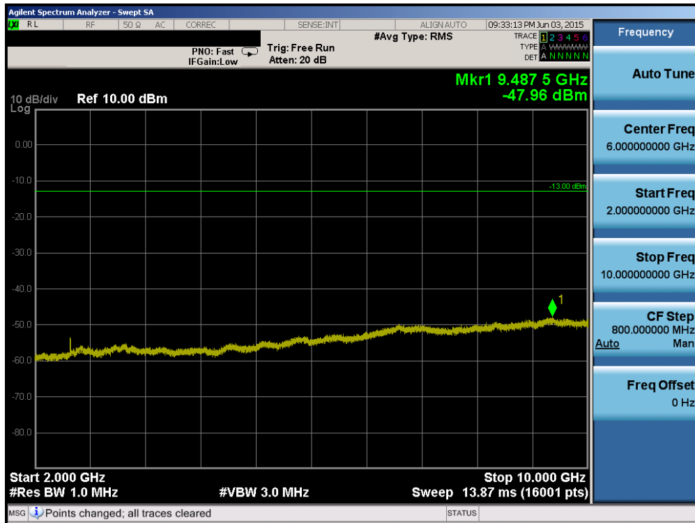
Plot 6-30. Conducted Spurious Plot (Cellular WCDMA Mode – Ch. 4183)
