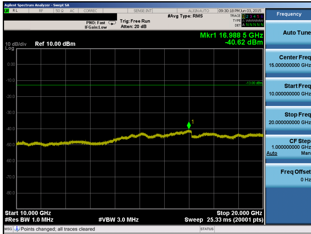
Plot 6-39. Conducted Spurious Plot (PCS WCDMA Mode – Ch. 9400)
