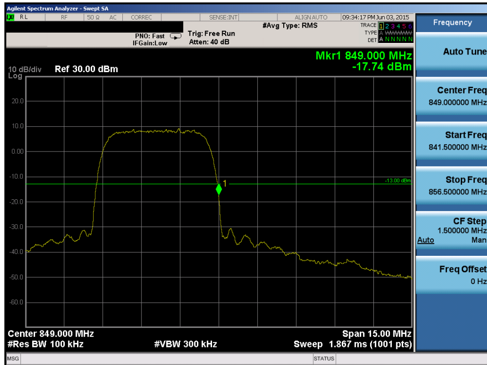
Plot 6-49. Band Edge Plot (Cellular WCDMA Mode – Ch. 4233)
