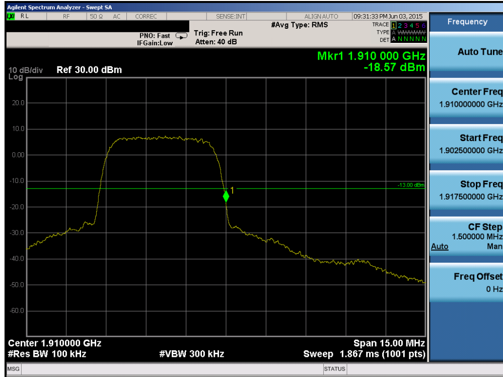
Plot 6-52. Band Edge Plot (PCS WCDMA Mode – Ch. 9538)
