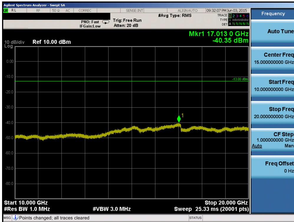
Plot 6-42. Conducted Spurious Plot (PCS WCDMA Mode – Ch. 9538)
