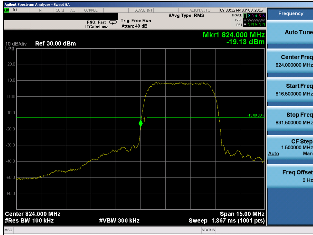
Plot 6-48. Band Edge Plot (Cellular WCDMA Mode – Ch. 4132)
