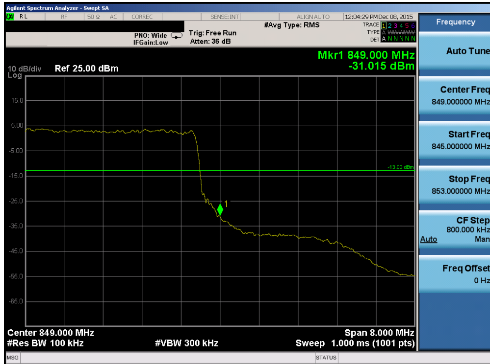
Plot 7-124. Upper Band Edge Plot (Band 5/26 – 10.0MHz QPSK – RB Size 50)
