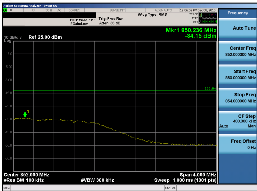
Plot 7-127. Upper Extended Band Edge Plot (Band 26 – 15.0MHz QPSK – RB Size 75)
