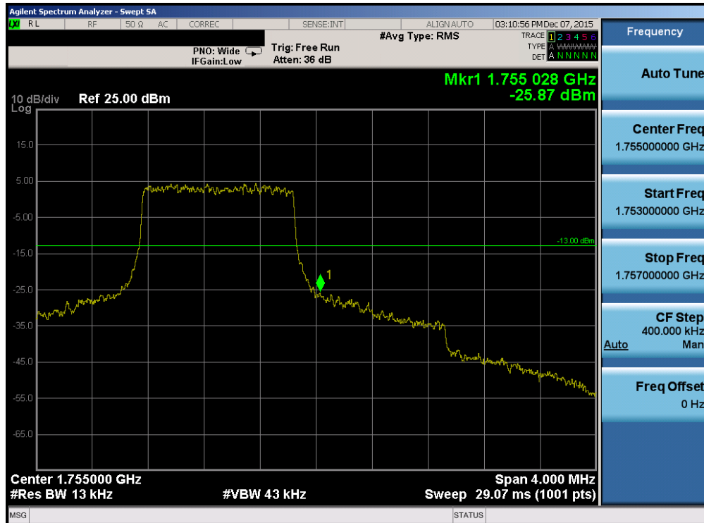
Plot 7-130. Upper Band Edge Plot (Band 4 – 1.4MHz QPSK – RB Size 6)
