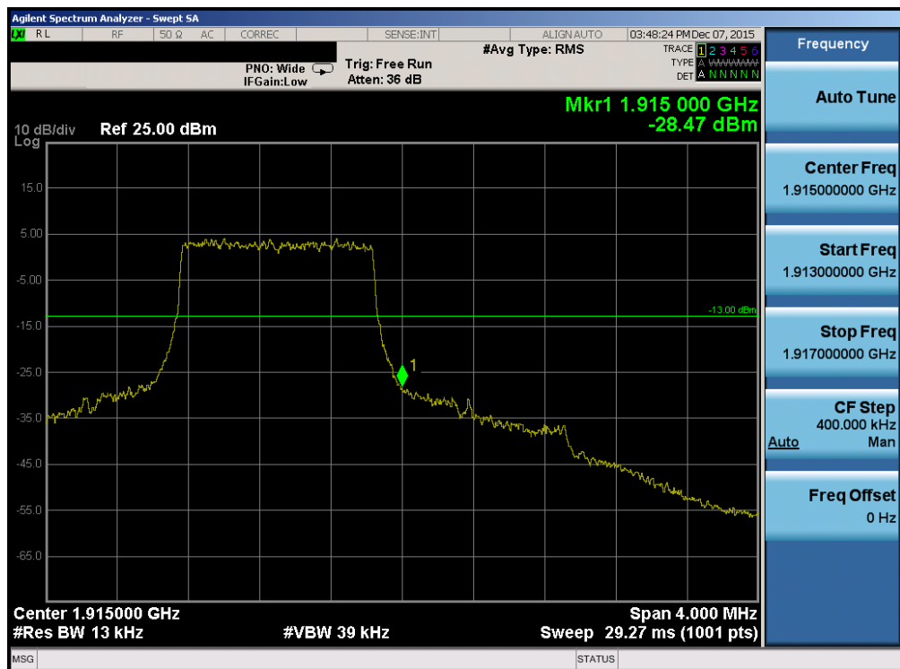
Plot 7-154. Upper Band Edge Plot (Band 2/25 – 1.4MHz QPSK – RB Size 6)
