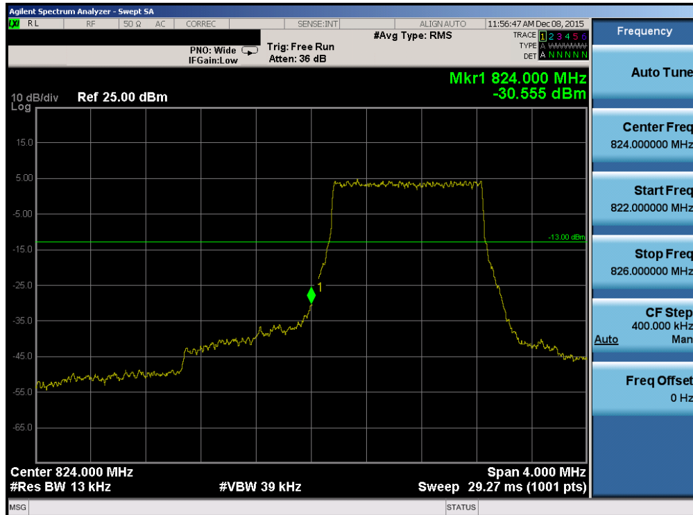
Plot 7-110. Lower Band Edge Plot (Band 5/26 – 1.4MHz QPSK – RB Size 6)
