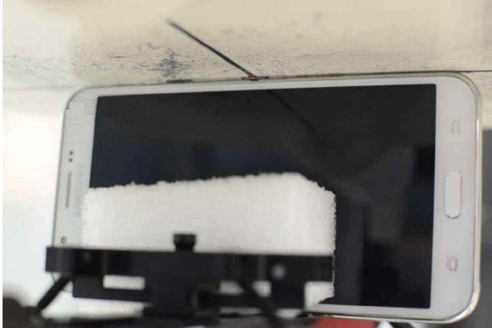
SAR Test Setup Photo 13 – Right Edge at 0 mm
