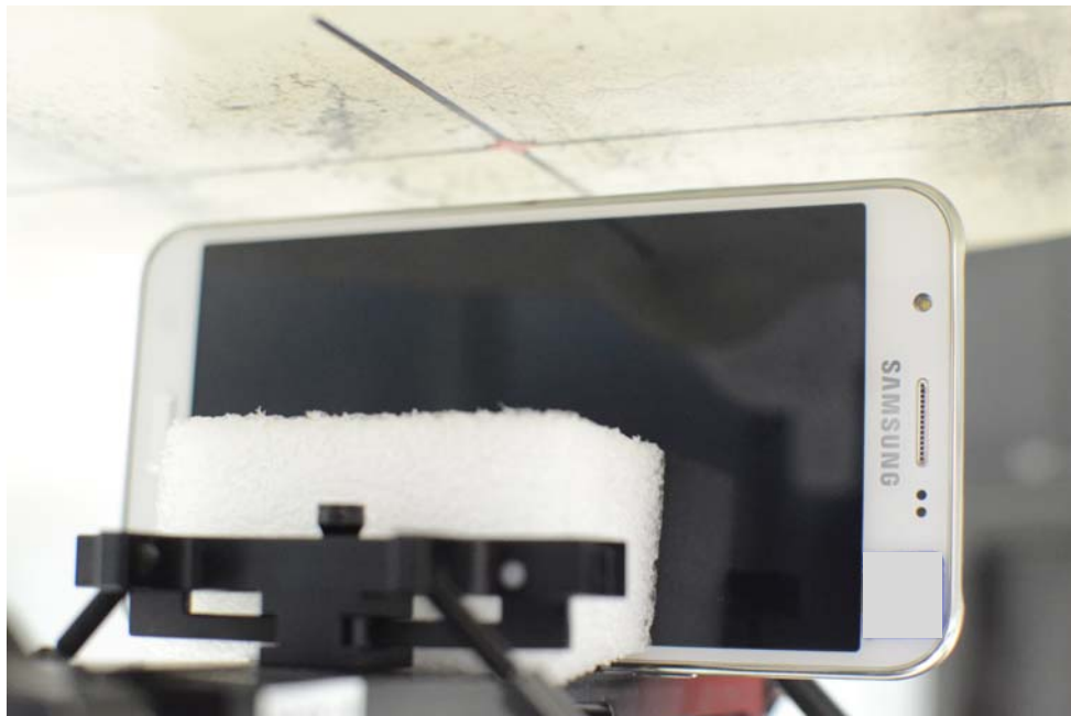
SAR Test Setup Photo 14 – Left Edge at 10 mm
