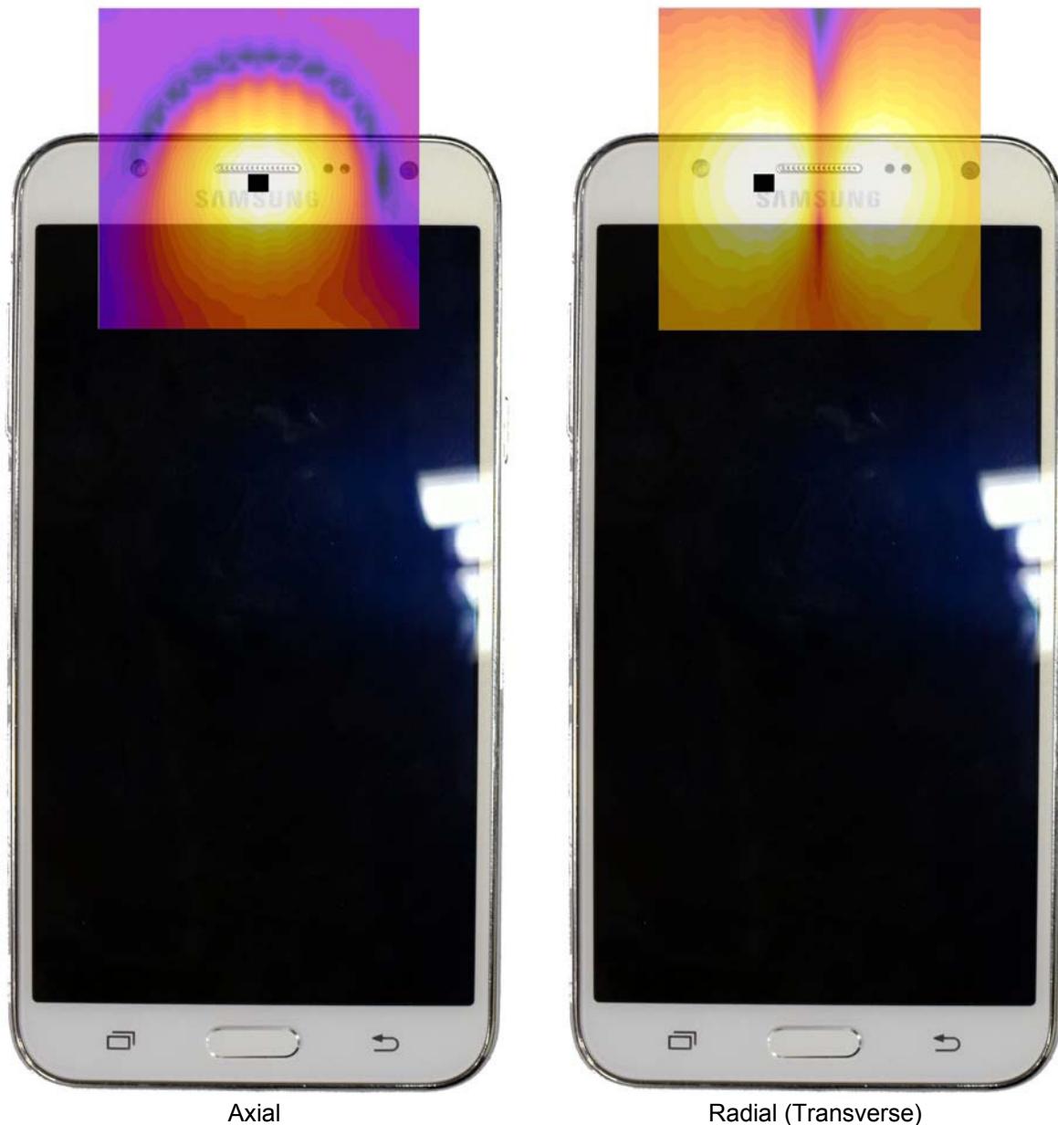
Axial Radial (Transverse) Figure 14-3 T-Coil Scan Overlay Magnetic Field Distributions
