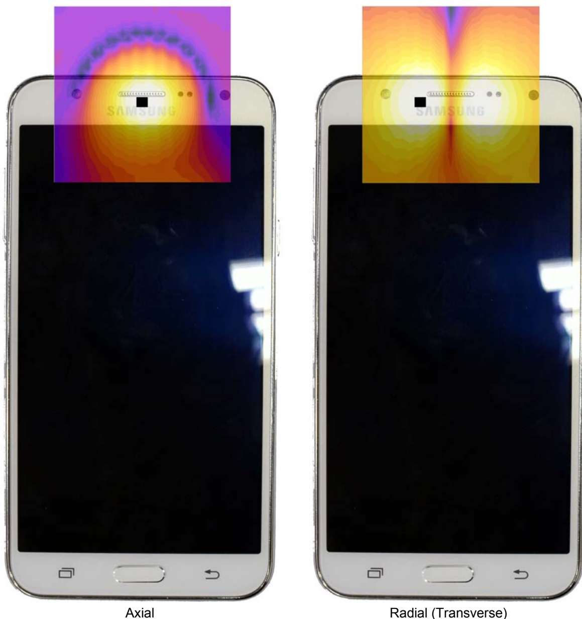
Figure 14-3 T-Coil Scan Overlay Magnetic Field Distributions
