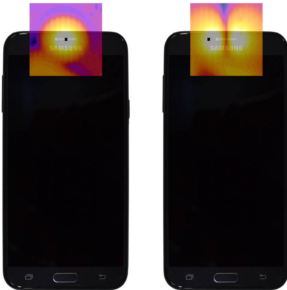
Figure 14-3 T-Coil Scan Overlay Magnetic Field Distributions
