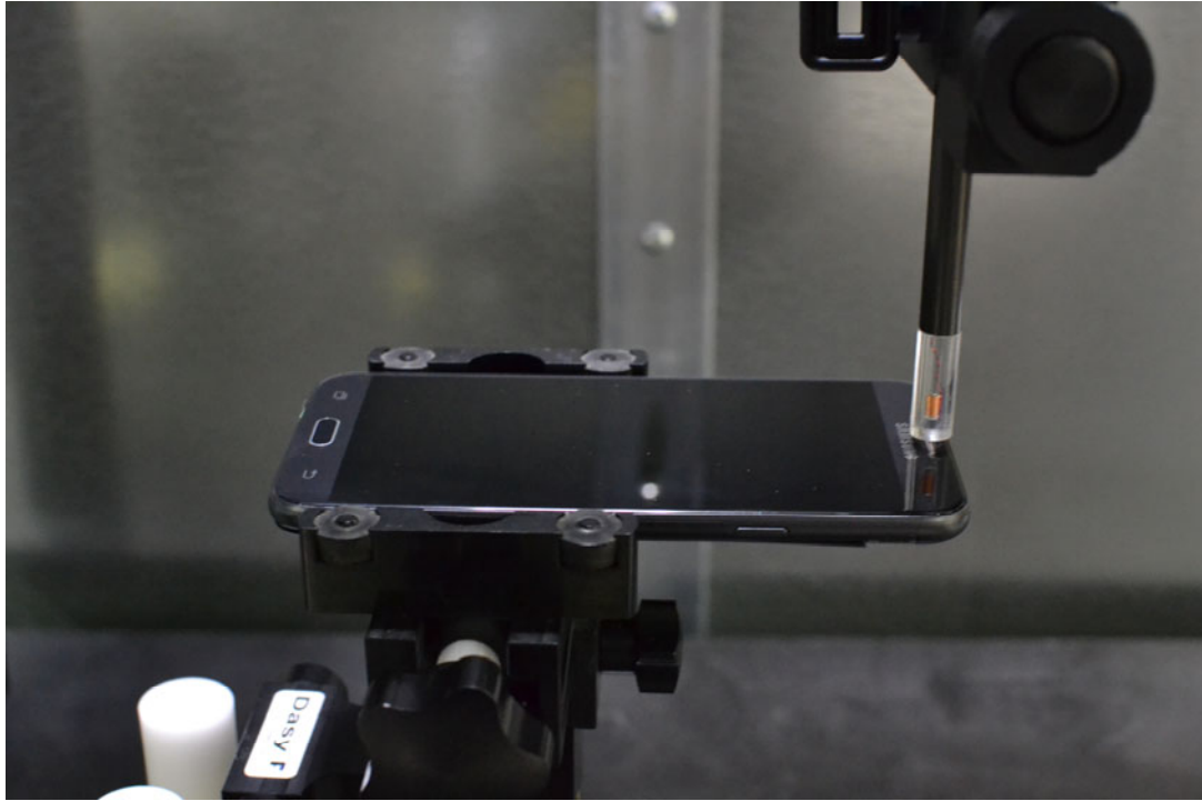
Figure 14-1 Test Setup for Wireless Device
