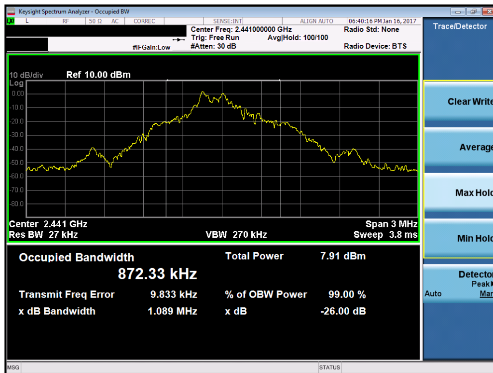
Plot 7-1. Occupied Bandwidth Plot (ANT+ – Ch. 39)
