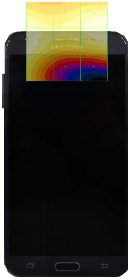
Figure 17-4 E-Field WD Scan overlay
