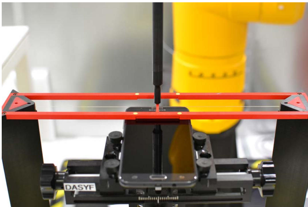
Figure 17-1 Ear Reference Point HAC Phantom Alignment
