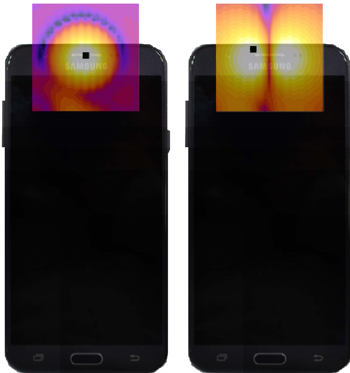
Figure 13-3 T-Coil Scan Overlay Magnetic Field Distributions
