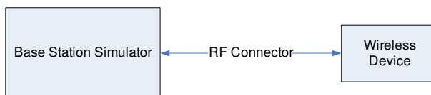
Figure 9-1 Power Measurement Setup
