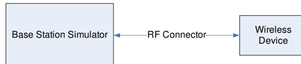
Figure 9-2 Power Measurement Setup
