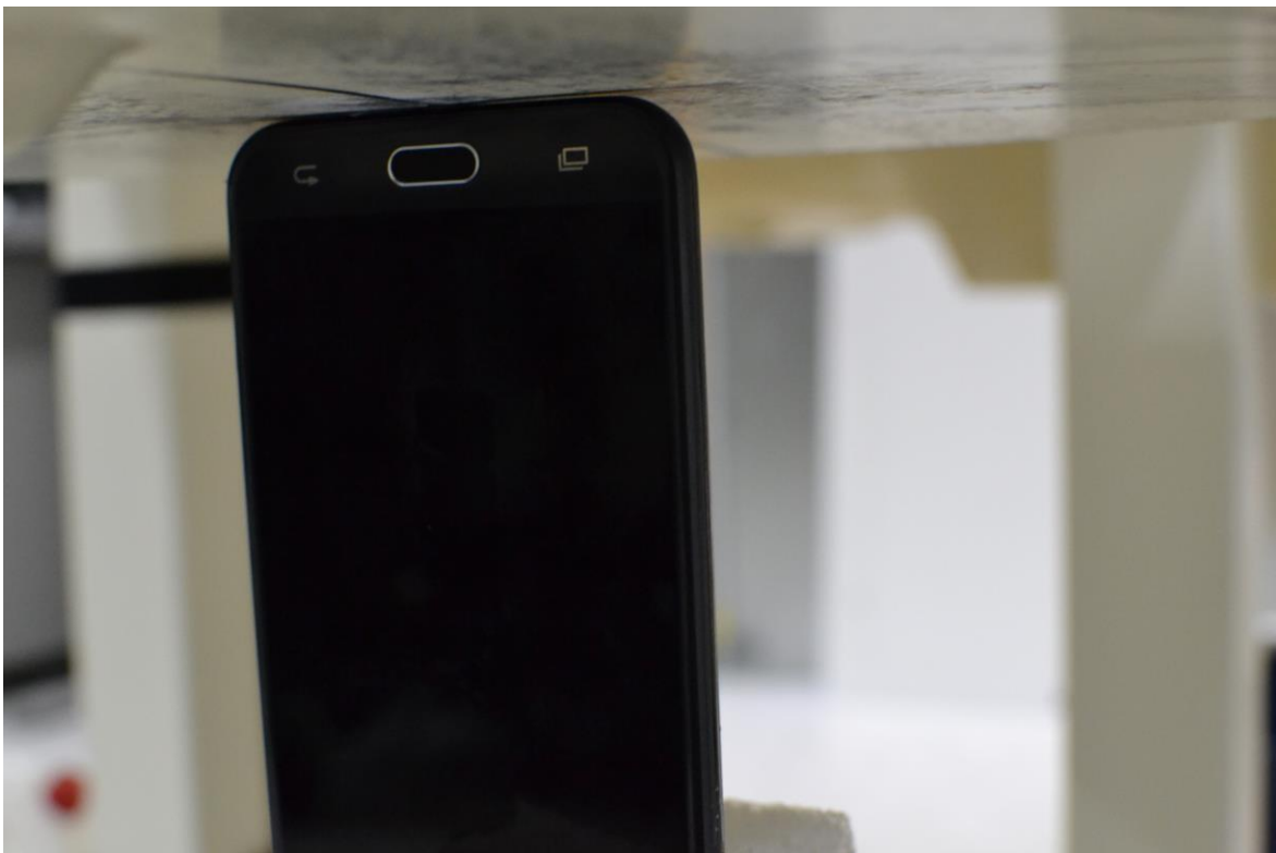
SAR Test Setup Photo 16- Bottom Edge at 0.0 cm (Phablet)
