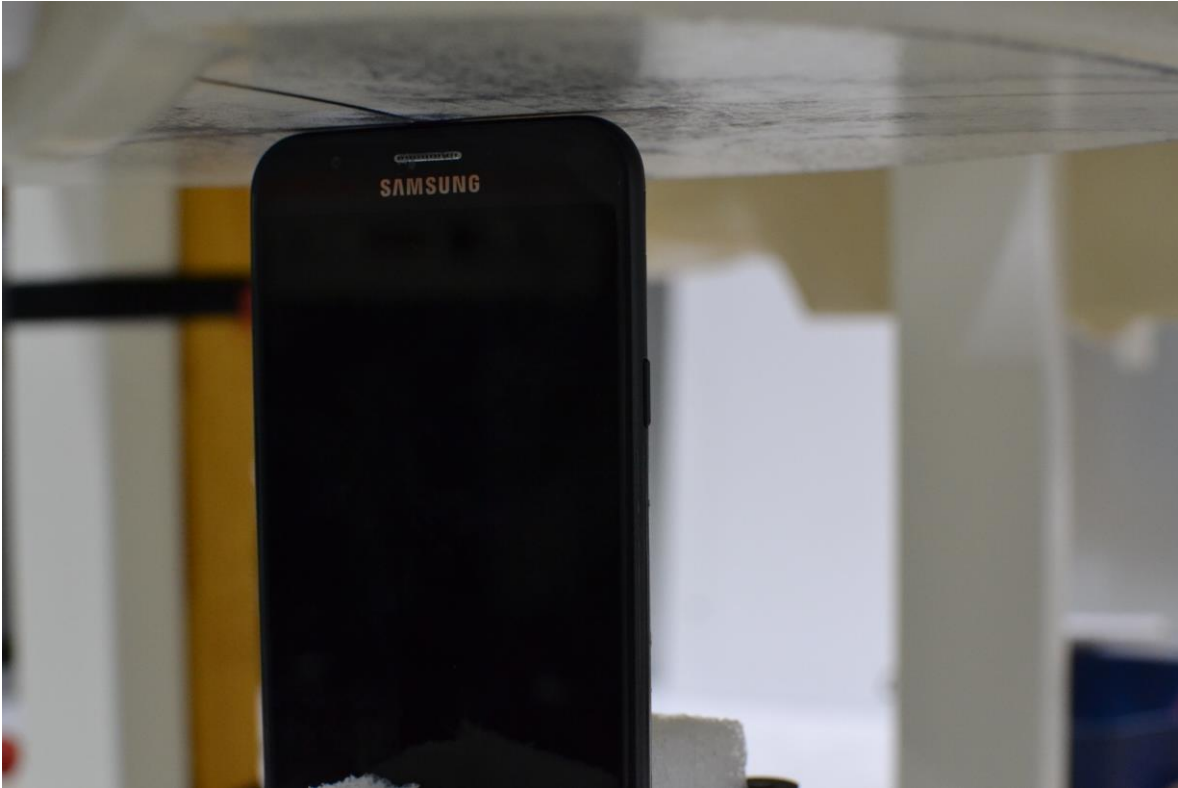
SAR Test Setup Photo 13- Top Edge at 0.0 cm (Phablet)
