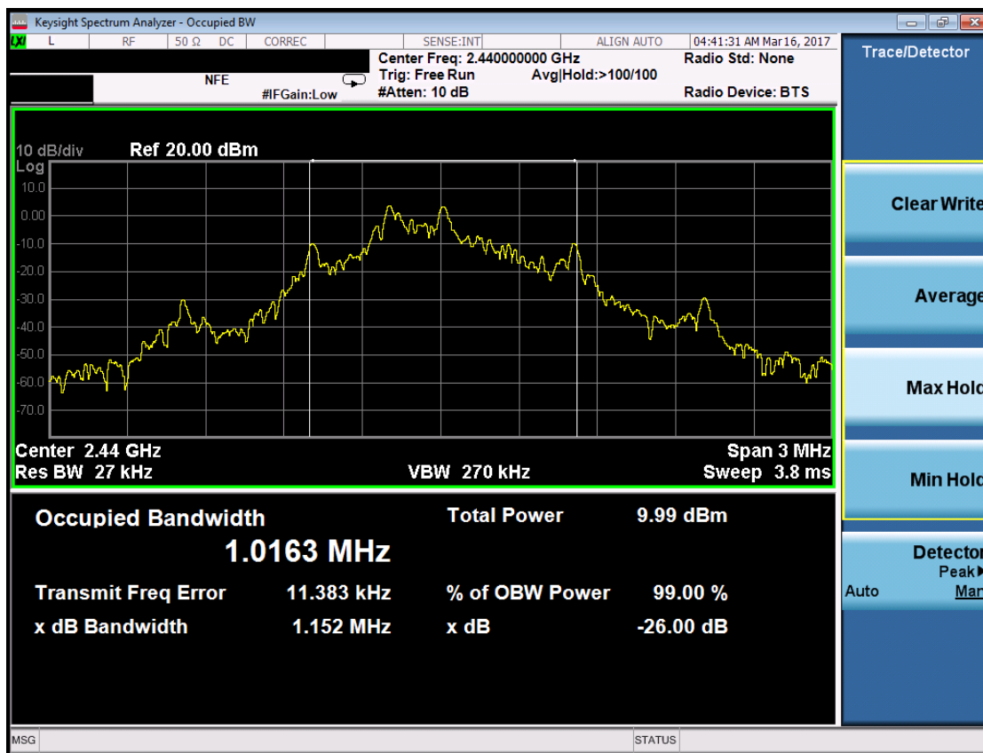
Plot 7-1. Occupied Bandwidth Plot (ANT+ – Ch. 38)
