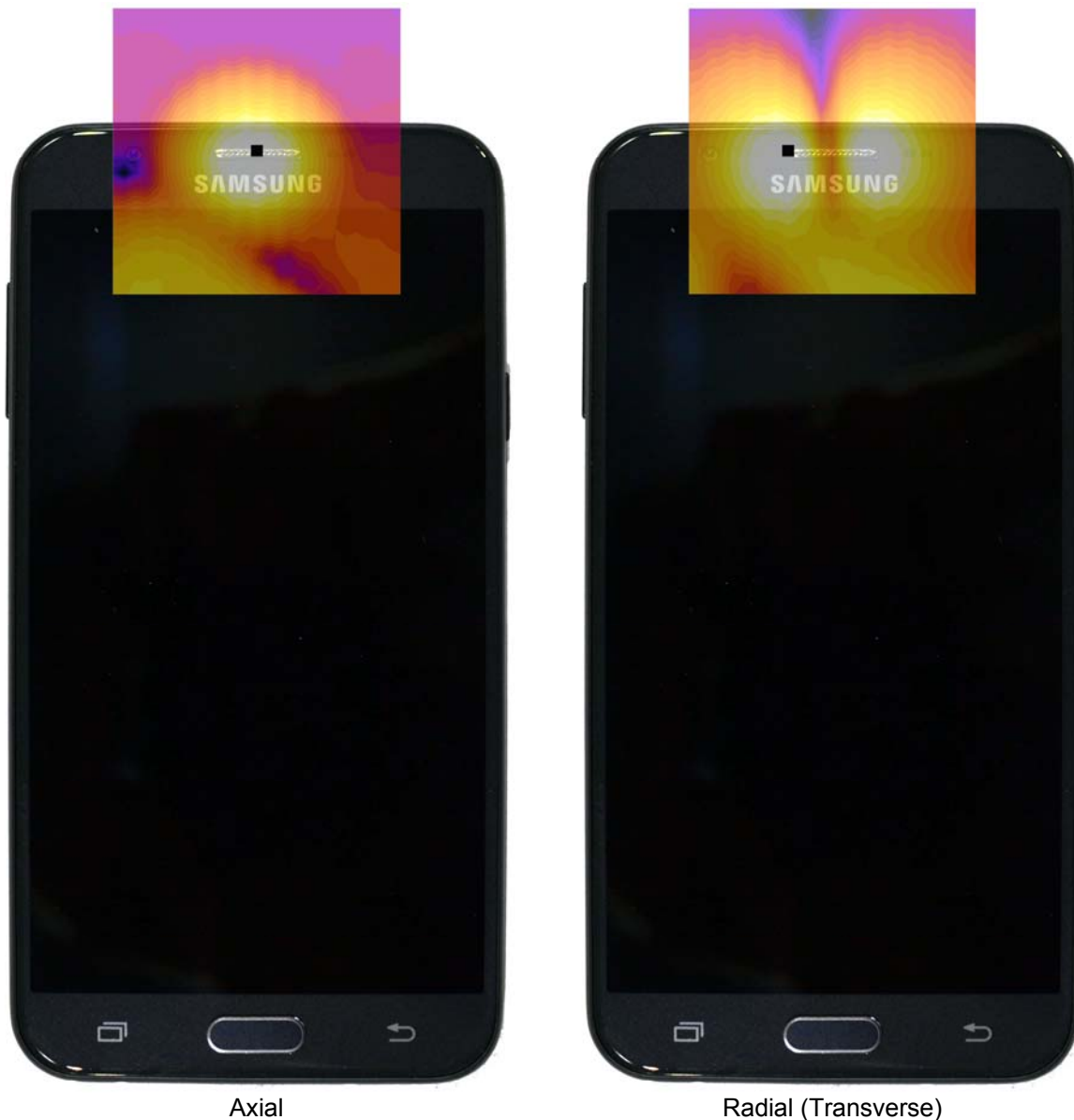
Figure 14-3 T-Coil Scan Overlay Magnetic Field Distributions
