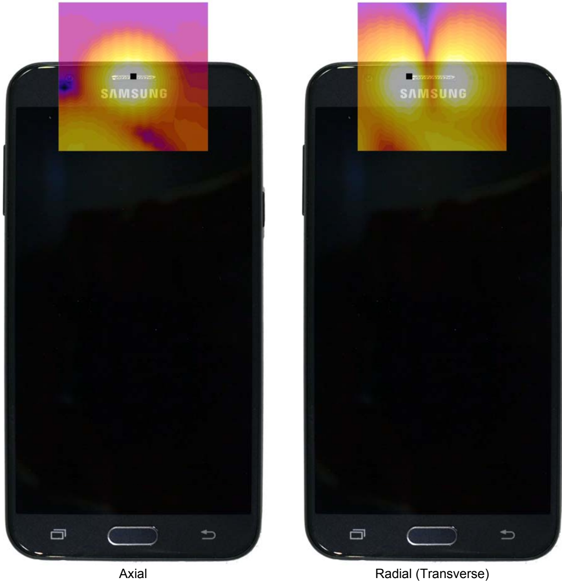
Figure 14-3 T-Coil Scan Overlay Magnetic Field Distributions
