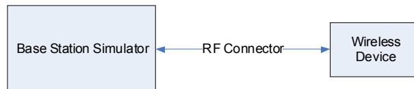
Figure 9-2 Power Measurement Setup
