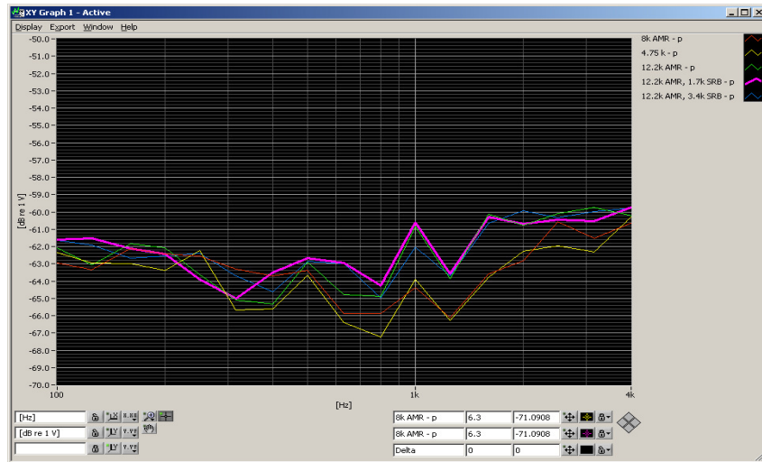
Figure 6-3 UMTS Audio Band Magnetic Noise
