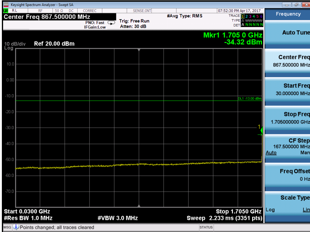
Plot 7-35. Conducted Spurious Plot (AWS WCDMA Mode – Ch. 1312)
