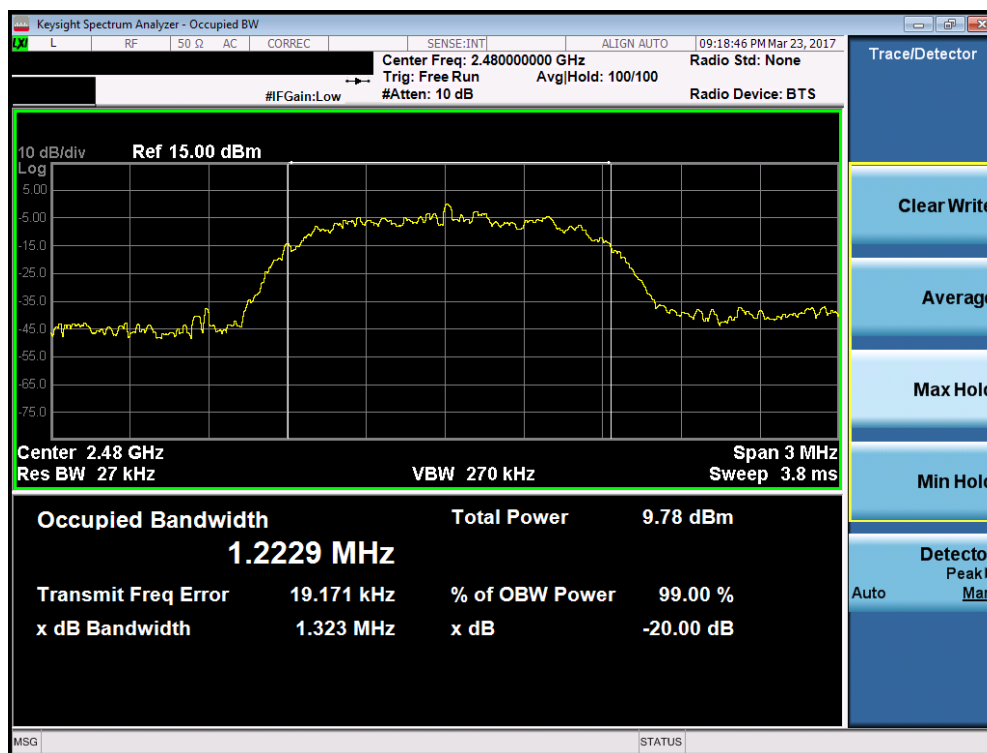
Plot 7-9. 20dB Bandwidth Plot (Bluetooth, 3Mbps – Ch. 78)
