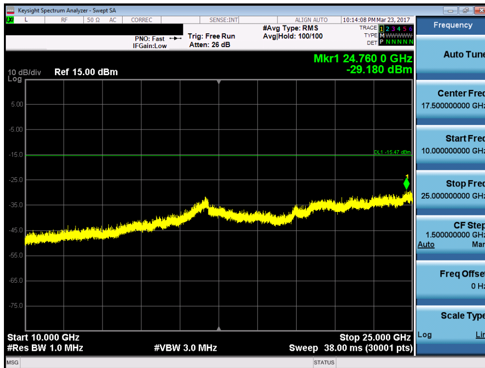
Plot 7-39. Conducted Spurious Plot (Bluetooth, 1Mbps – Ch. 39)
