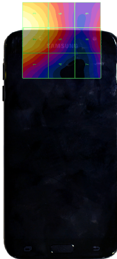
Figure 17-4 E-Field WD Scan overlay
